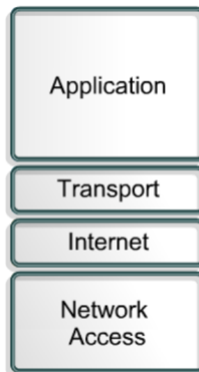
Figure 11: - TCP/IP Reference Model
